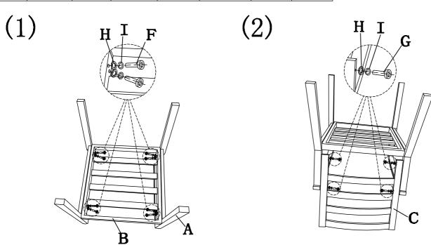
Please do not tight the screw until all screws lined up with holes and try to tight it loosely initially in all screws then tight a little bit more in all screws. Do not overtight one screw that will make other screws hard to tight but tight all screws firmly in the end.
