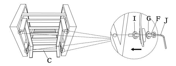
Please do not tight the screw until all screws lined up with holes and try to tight it loosely initially in all screws then tight a little bit more in all screws. Do not overtight one screw that will make other screws hard to tight but tight all screws firmly in the end.
